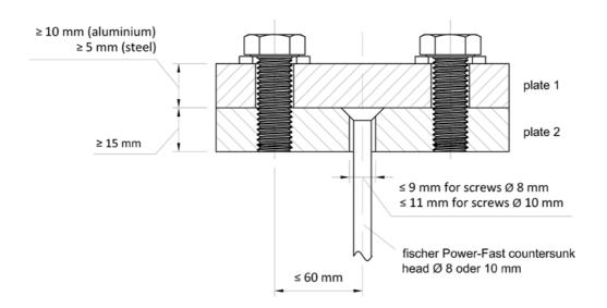
Information for the structural analysis of the metric screw connection and the metal plates are not part of this European Technical Assessment.
