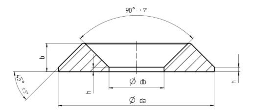
Washer for Power-Fast and construction screws
